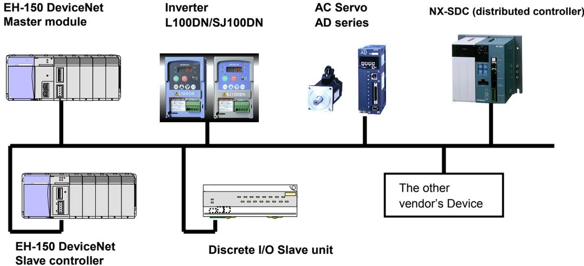
Figure 2.1 Hitachi made DeviceNet products
