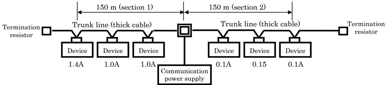
Total power consumption value of section 1 = 1.4 A + 1.0 A + 1.0 A = 3.4 A
