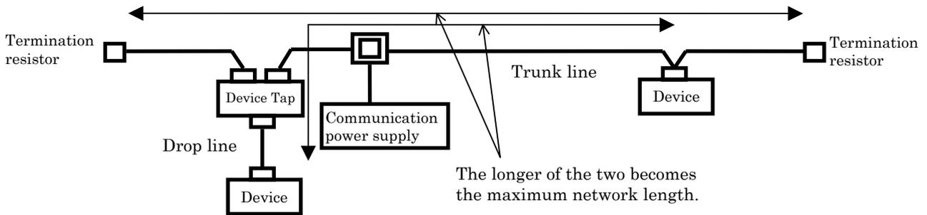
The communication cables in the network can be either of the two types: thick cable (trunk cable) or thin cable (drop cable).
