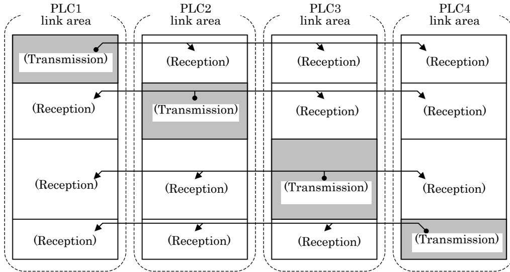
Figure 9.3 Link area in the H series CPU link
