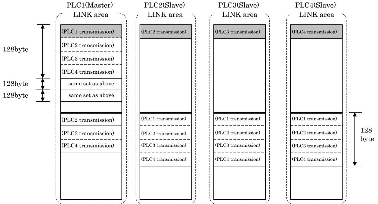
Figure 9.5 LINK system with slave mode (Example)
