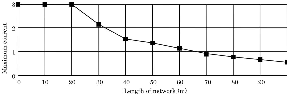
Figure 12.2 Maximum current capacity (thin cable)
