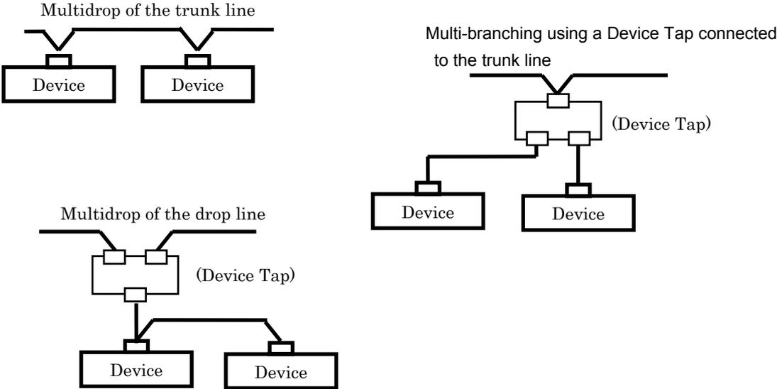
Figure 2.2 Connection methods for DeviceNet
