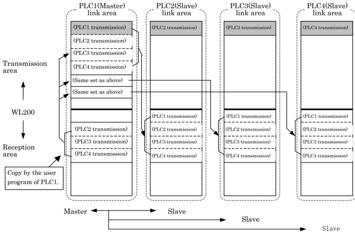
Figure 9.4 Link system using the slave mode
