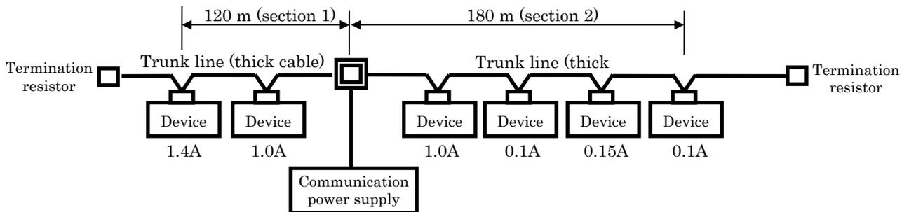
Total power consumption value of section 1 = 1.4 A + 1.0 A = 2.4 A
