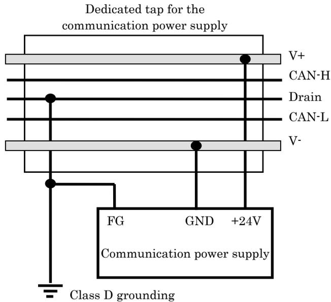
If two or more communication supply units are used, only one of them should be grounded with the shielding line. Furthermore, do not connect other communication power supply units with the shielding line.
