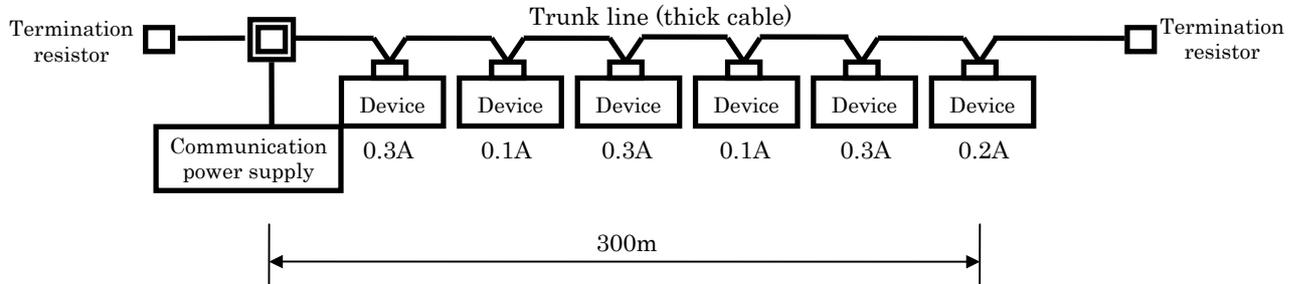
Total power consumption value =  $0.3 \text{ A} + 0.1 \text{ A} + 0.3 \text{ A} + 0.1 \text{ A} + 0.3 \text{ A} + 0.2 \text{ A} = 1.3 \text{ A}$
