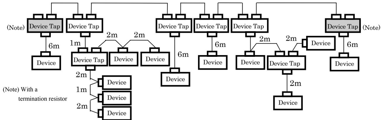
In the configuration example above, the length of each drop line is within 6 m and causes no problem, but the total length of all the drop lines becomes 42 m. This is longer than the restriction on the total drop line length of 39 m at a communication speed of 500 kbps. Therefore, a communication speed of 125 kbps or 250 kbps should be used.
