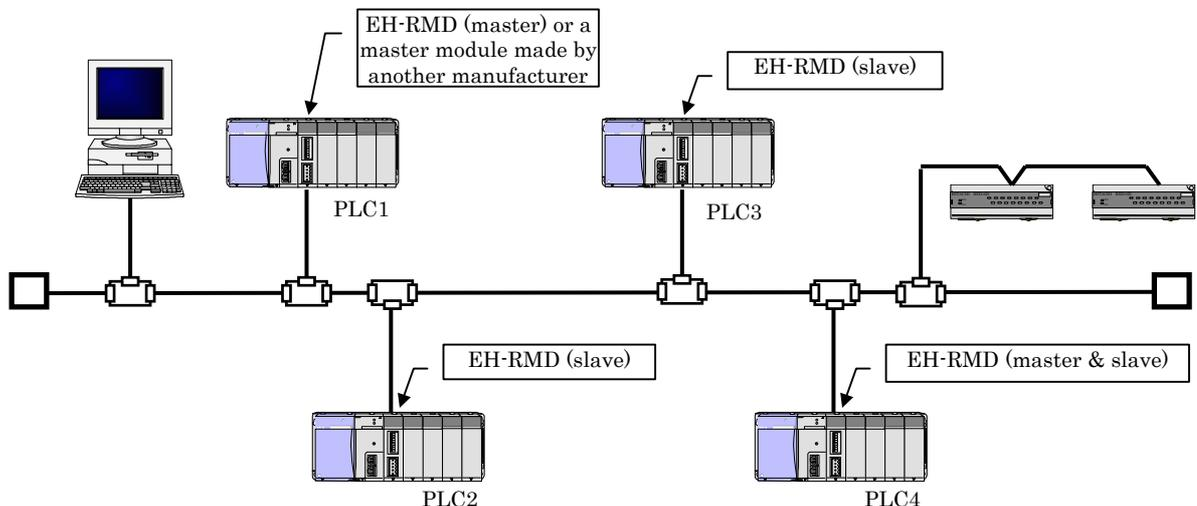
Figure 9.2 System configuration example 2 illustrating the use of the slave mode
