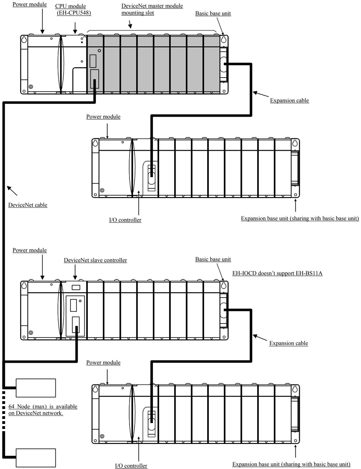
Figure 3.1 EH-150 system configuration diagram (ex. Using EH-CPU548)
