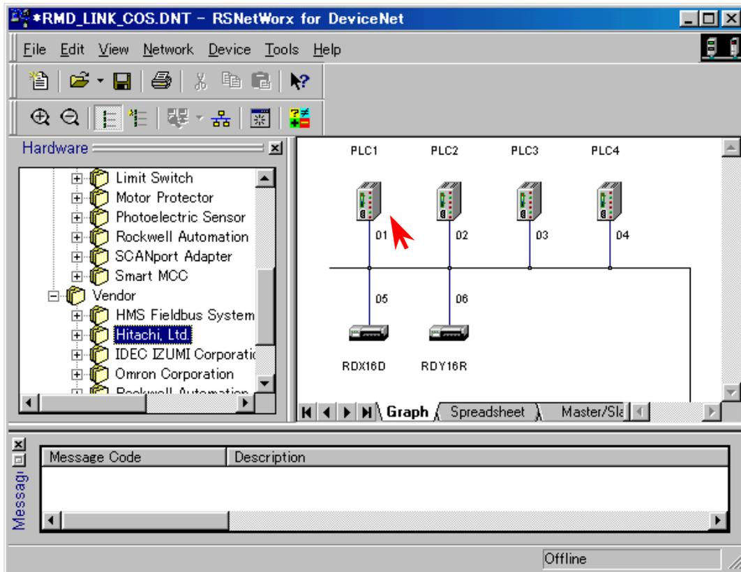
Display the **[Scanlist]** tag, and move the devices from Available Devices to Scanlist. Click **[Edit I/O Parameters]** for each of the devices moved to Scanlist and check the I/O data size. It is possible to view the information of each slave set in Step 1.
