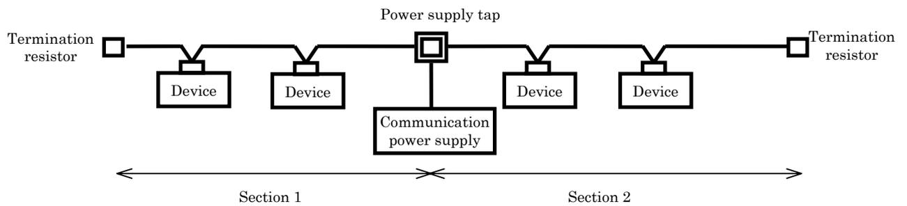
The single power supply central connection allows supplying a total power capacity twice that of the single power supply termination connection.
