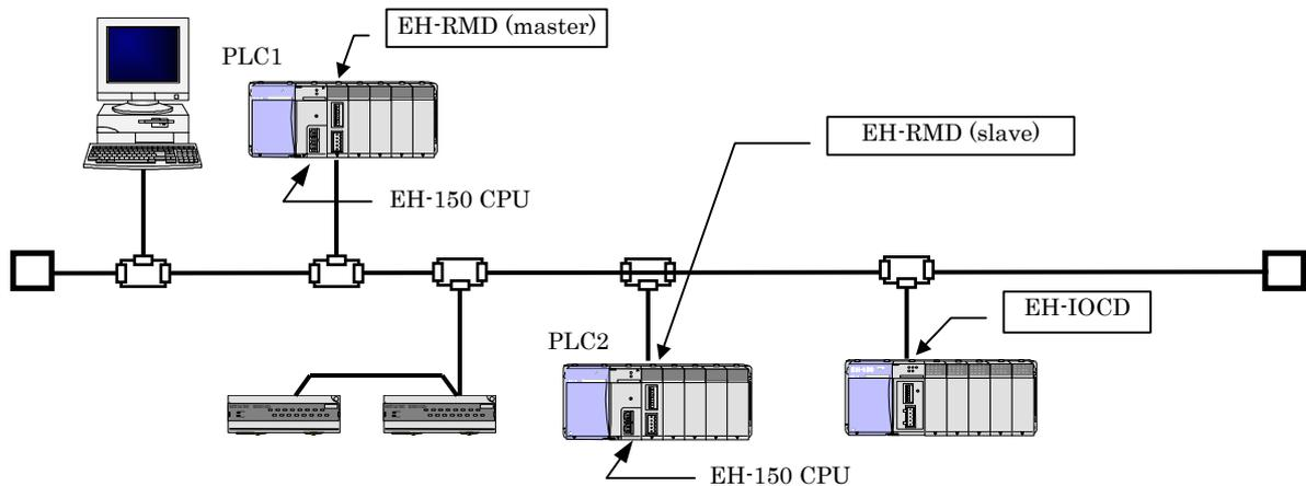
Figure 9.1 System configuration example 1 illustrating the use of the slave mode
