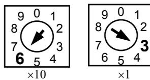
Figure 7.1 Setting the Node Address
