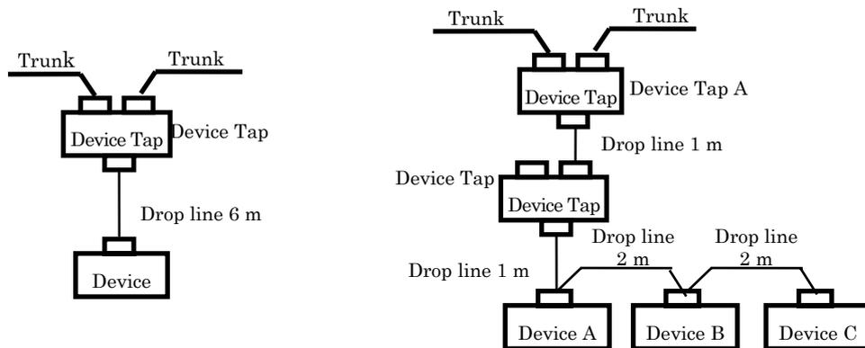
2 m from Device Tap A to device A
