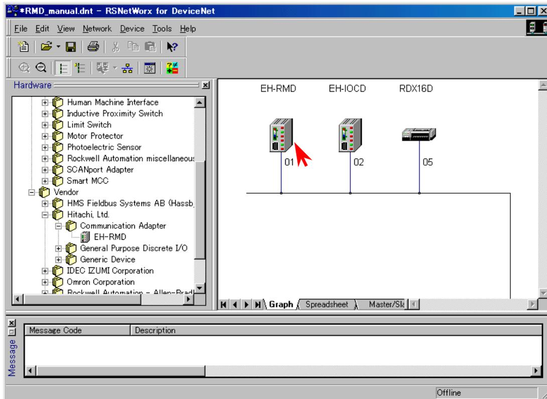
Click the **Scanlist** tag and move the device from **Available Devices** to **Scanlist**. Highlight each device moved to Scanlist and click **[Edit I/O Parameters]**. Set the I/O communication type and I/O data size.
