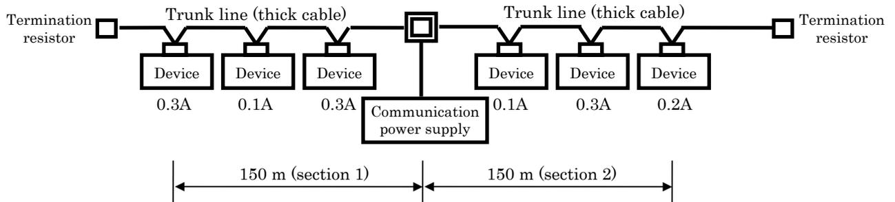
Total power consumption value of section 1 =  $0.3 \text{ A} + 0.1 \text{ A} + 0.3 \text{ A} = 0.7 \text{ A}$
