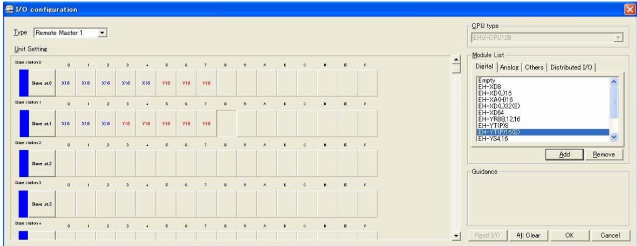
Figure 4.30 Example of I/O assignment for slave bases (with Control editor in system configuration example-14)
