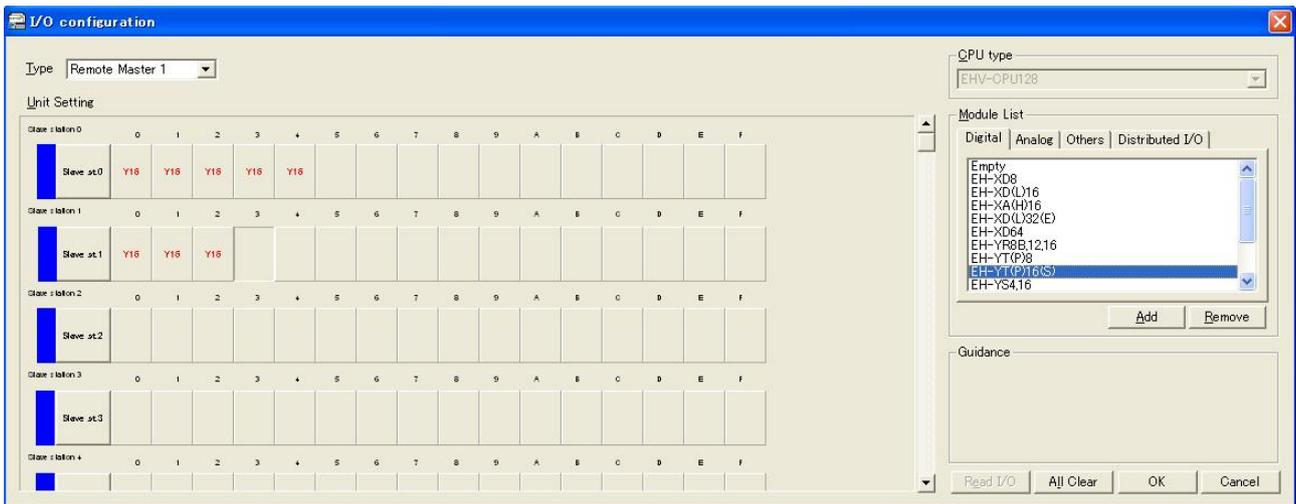
Figure 4.23 Example of I/O assignment for slave bases (with Control editor in system configuration example-8)
