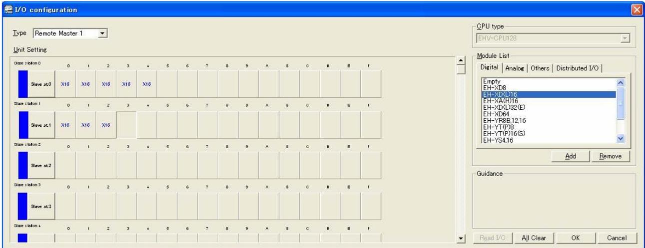
Figure 4.27 Example of I/O assignment for slave bases (with Control editor in system configuration example-12)
