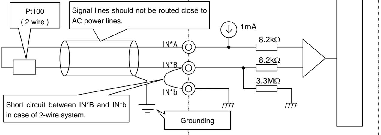
\* 3-wire system is recommended for this product. Since cable resistance is not cancelled in 2-wire system, it is not suitable for high accuracy measurement especially for long cable used.
