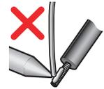
Wire the stripped cable after twisting it to prevent it from becoming loose. In addition, do not solder it.
