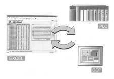
The device data in the PLC can be monitored inreal-time with Excel, and recipe data in Excelcan be transfered to the PLC.
