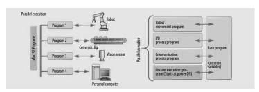
Multitasking function for parallel execution of multiple tasks
