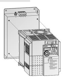
Installing an EMC noise filter on an FR-F700
