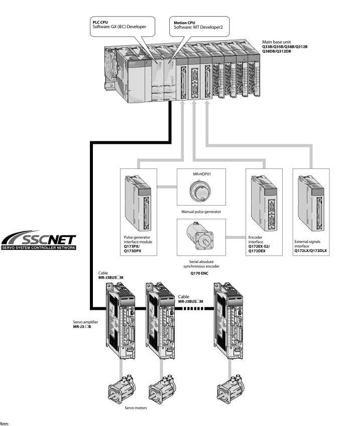
The first CPU on the main base unit must always be a PLC CPU (e.g. Q00, Q01, Q02/Q02H/Q06H/Q12H/Q25H/QnUD(H) Serie).
