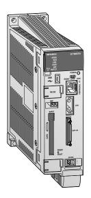
The Q170MCPU combines a PLC CPU, a Motion CPU and a power supply module into one compact unit. No base unit is required, although an extension base unit with standard PLC modules can be connected if required. An encoder interface is included as standard, enabling multiple axis synchronization with an external encoder.
