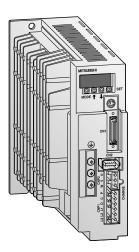
The servo ampflifier of the series ME-E Super combines unique functions with very compact dimensions. With its high positioning accuracy and high responsivness the MR-E Super is suitable for applications from 100 W to 2 kW. Availible functions of the drive are e.g. position/internal speed control mode, speed/torque control mode and Mitsubishis well known real-time auto-tuning. The compact size helps designers, to fit all control components needed for an automation system into the smallest space.
