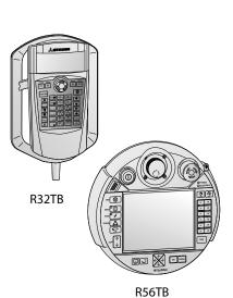
The R56TB teach panel is a multifunctional control and programming terminal for all Mitsubishi SD series robots. Its intuitive user interface makes it easy to control robot movements and perform extensive diagnostics and monitoring functions for users of all levels. All safety-critical functions such as robot movements are assigned to keys. Programming and monitoring functions are
