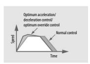
Automatic acceleration and braking ramp optimisation for faster cycle times
